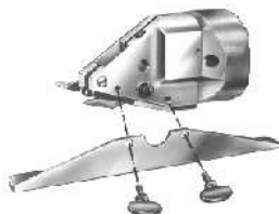
assembling side guide with two wing screws
