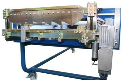
detail picture of guillotine shear (K1-QB) with electric motor (K1-EUQB). Picture without cover.
