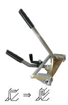
Hand Seamer for Double Lock, K7-1: closes the pre-closed standing seam in one operation into a double lock seam.
